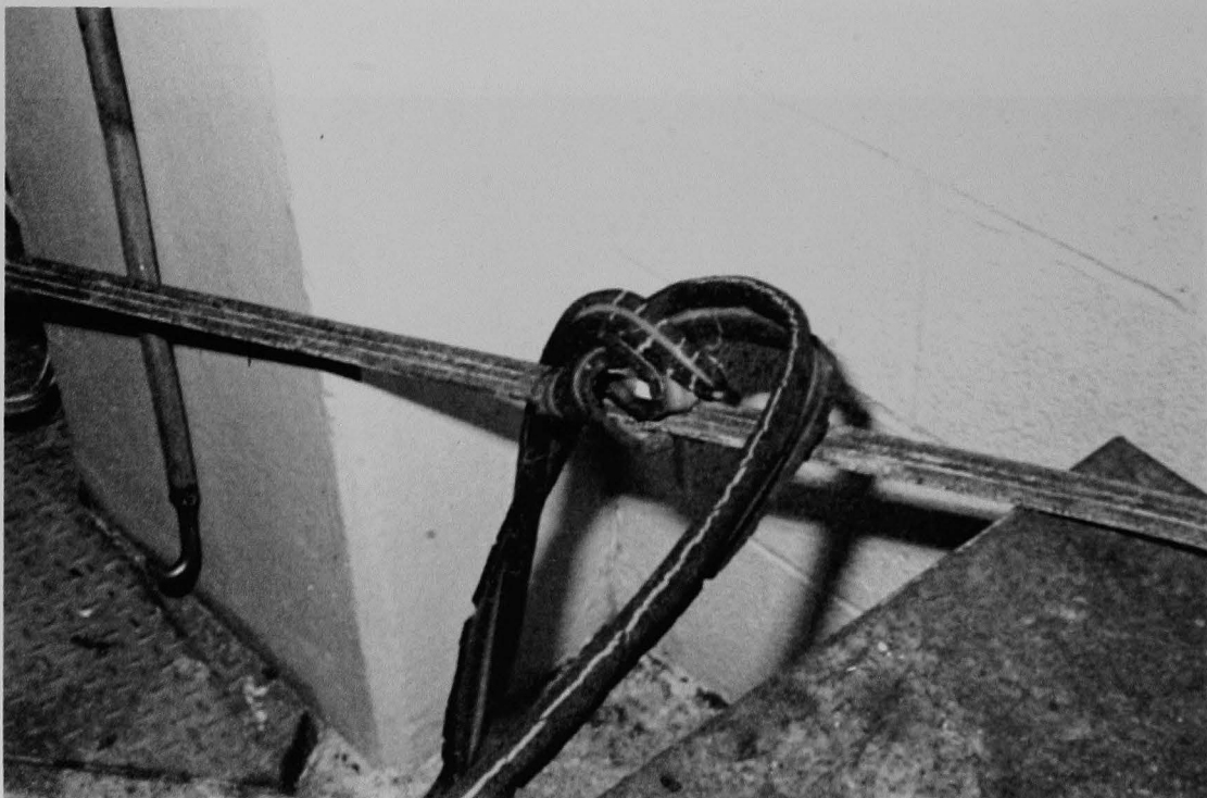
Figure 120 (4). Crane power cable and insulation lying over tool box south of enclosed stairwell (see Figure 119).
